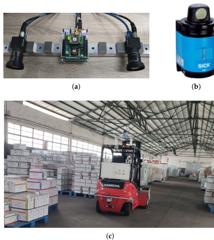
Figure 4. Dataset collection platform that includes the stereo camera, NAV350 laser sensor, artificial reflective landmark, and automatic guided forklift. (a) Stereo camera. Two monocular cameras triggered by the same signal source were used to capture pictures of the warehouse. (b) SICK NAV350. The NAV350 sensor was used to measure the global position of the forklift in the warehouse. (c) The forklift running in the warehouse.
