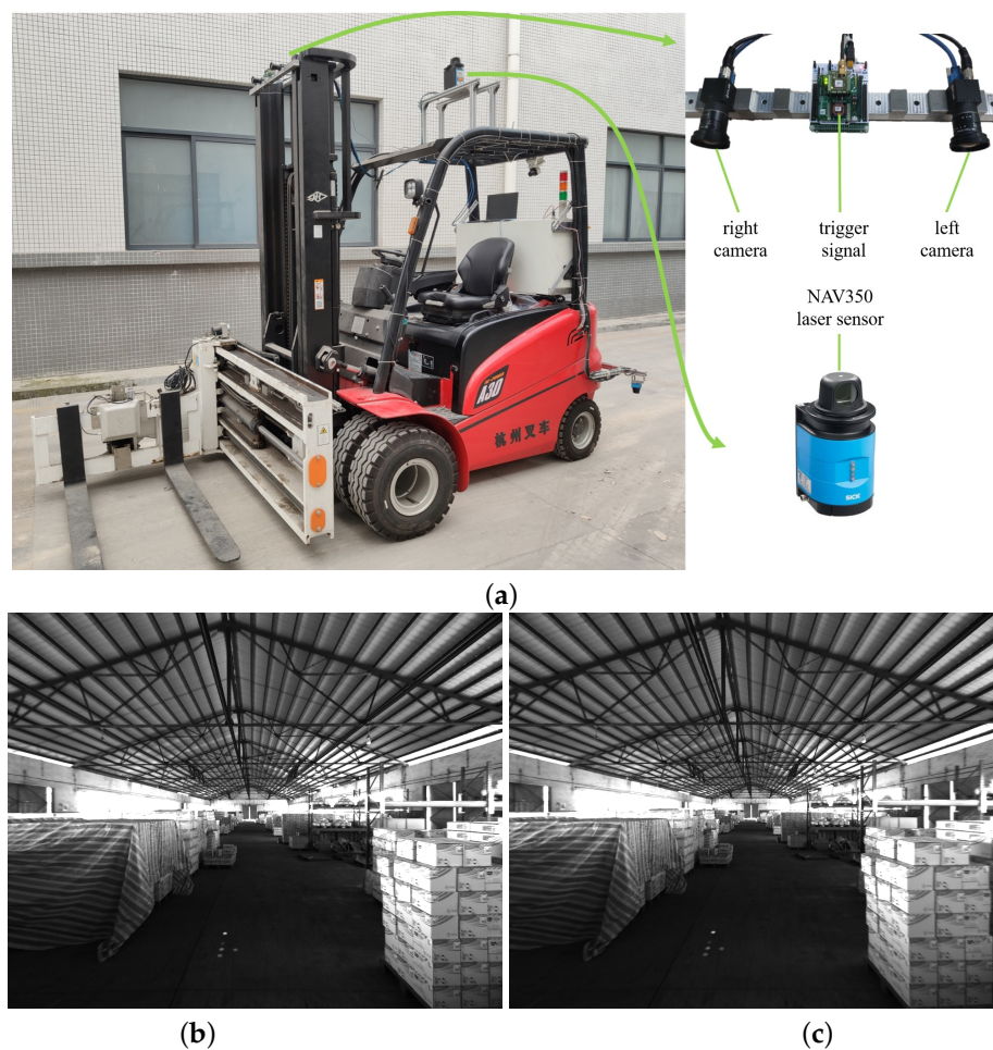
Figure 2. The forklift equipped with basic sensors in our proposed system. (a) Two monocular cameras triggered by the same signal source are used to capture pictures of the warehouse, and the NAV350 sensor is used to measure the global position of the forklift in the warehouse. (b) The image captured by left the monocular camera; (c) the image captured by the right monocular camera.
